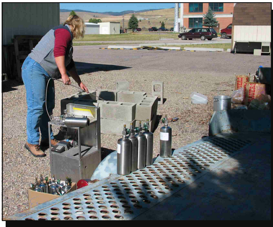
Figure 2—Using canisters to collect gas samples from a simulated campfire for analysis with a gas chromatograph-mass spectrometer.
