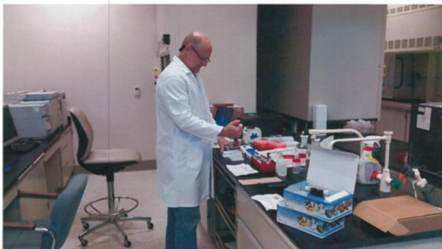
Gerry Morford (Technical Services Section – Environmental Scientist V) loads an ELISA plate counter for HAB - Microcystin analysis.
