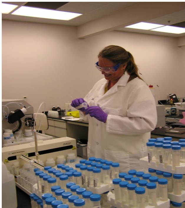
JoEllen Thompson (Metals Section) loads the autosampler on an Inductively Coupled Plasma Mass Spectrometer (ICPMS) instrument with DOW water samples for analysis.
