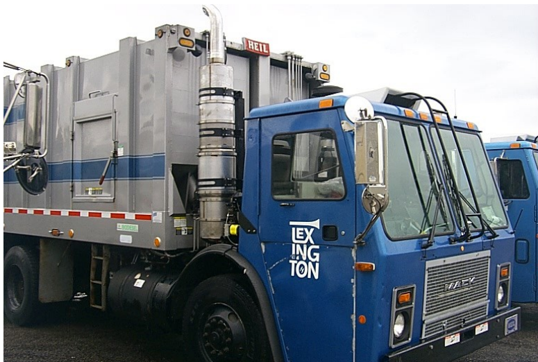
The Lexington-Fayette Urban County Government utilized Clean Diesel Grant Program funding to retrofit 12 garbage trucks with diesel particulate filters. Louisville Metro Government completed similar retrofits of 20 garbage trucks using grant funding through DAQ's Clean Diesel program.
